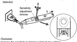
Increase the sensitivity to detect a relatively low voltage. Counterclockwise:
